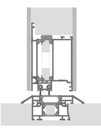
The Alta+ threshold ensures high durability and effective waterproofing. Additionally, the Alta+ is engineered to facilitate smooth mobility, ensuring easy movement in and out.
