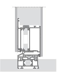
The Alta threshold is crafted to withstand harsh conditions while maintaining a sleek, sophisticated appearance. It's perfect for projects that require a high level of durability and effective waterproofing without sacrificing visual appeal.
