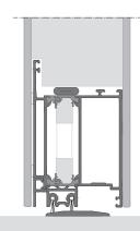
The Mida threshold provides a solid, robust option that excels in both performance and durability. Its design ensures excellent waterproofing, making it suitable for areas where weather resistance is needed without compromising on style.
